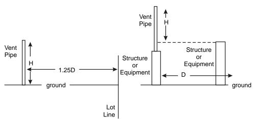
H = Minimum height in feet of vent pipe above the ground or above any structure or equipment within distance (D) where personnel might be present.
